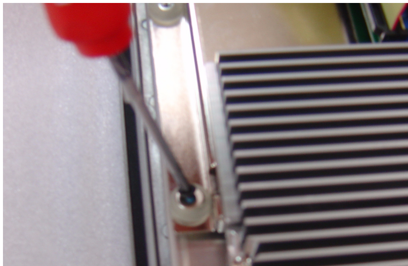
Figure E.14: Fastening the HDD Module
