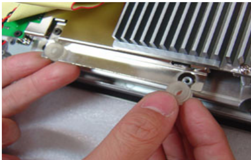
Figure E.3: Removing the HDD kit
