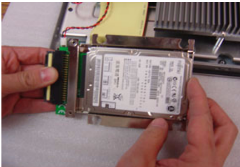
Figure E.6: Installing the HDDr
