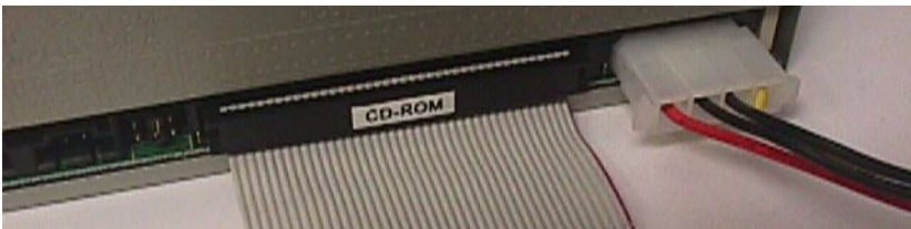
Figure D.7: Plug Power Line into CD-ROM Drive
