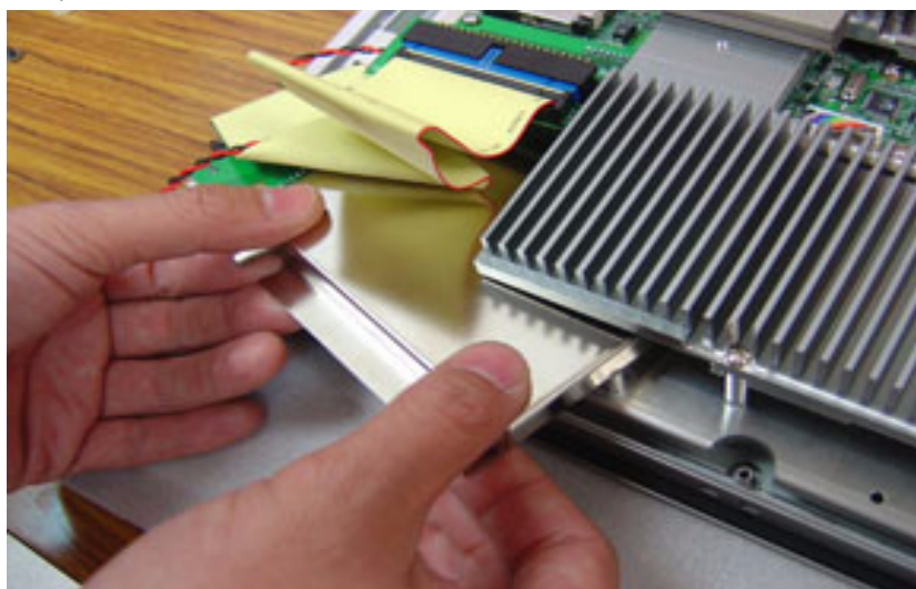
Figure E.4: Pulling out the HDD bracket
