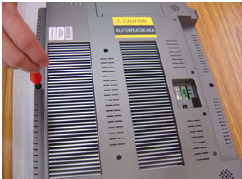
Figure E.15: Reinstalling the Rear Cover
