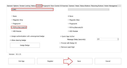
Once the card reader is set up, assigning badges can be done in the same place by pressing the "Assign Badge" button. Then select an ElOBoard user from the dropdown above and select "Assign Badge". Next present the badge to be associated with that user. This badge is now assigned and will be used to change the user status.
